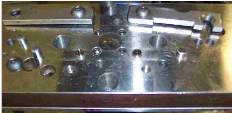
Figure 28: A fixture used in for creating lap SFW welds.
