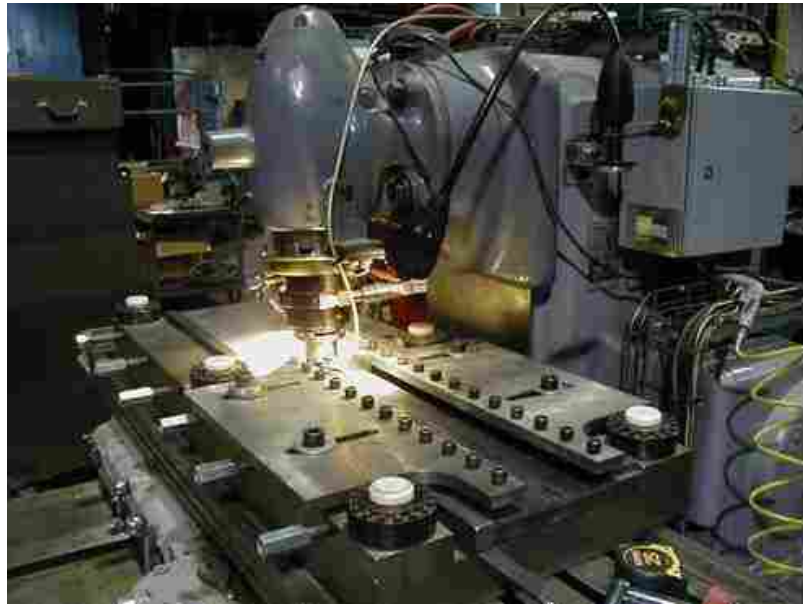
Figure 26: Friction stir weld machine used in this study.
