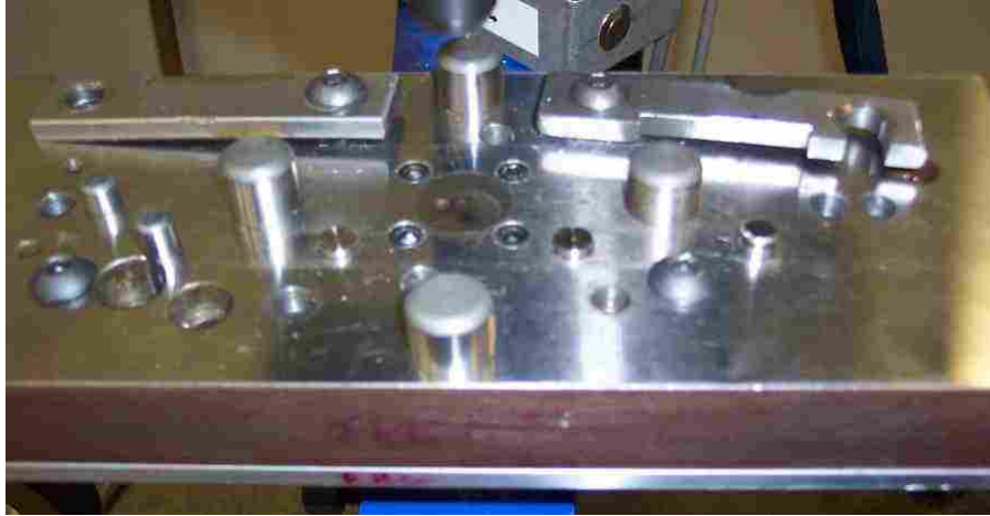
Figure 27: A fixture used in this study for creating cross tension SFW welds.
