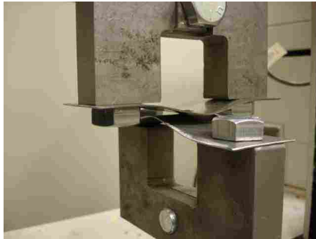
Figure 25: The cross tension pulling fixture used in this study.
